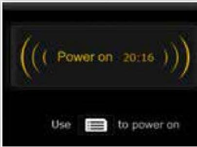
Touch the [Menu Key] key to confirm you want it to turn on. When your BIBO switches back on from the 'Power on/off' mode, the hot tank will take approximately 5 minutes to heat back up to the maximum temperature and the cold tank will take approximately 15 minutes to chill back down to the minimum temperature.
