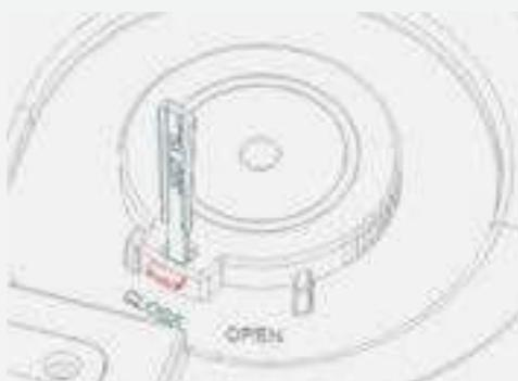
Remove the UV lamp from its packaging and insert it carefully. Then rotate clockwise until it clicks and locks.
